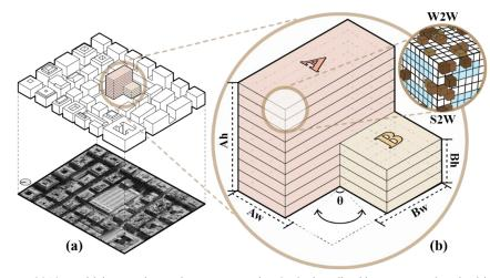
Figure 2 (a) Proposed building site in Genoa, Italy and (b) The building form and relevant design parameters
