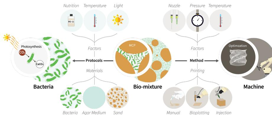
Fig. 1. Diagram, Research workflow for adapting the biomixture to both the bacteria and the machine through environmental, material and fabrication parameters.
