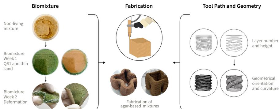
Fig. 3. Diagram, Implementing the pre-fabrication phase towards the second phase of the co-fabrication workflow. (Right) Developing the biomixture and examination of biological activity. Comparison of spatial cell distribution within QS1 and thin sand. (Left) Developing a potential printing tool path and geometrical properties. (Middle) Initial 3D printing experiments with agar-based mixtures for examining agar adhesion and structural integrity.
