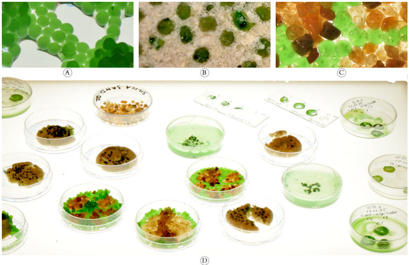
Figure 5. Compositional and geometric variations in early-stage material experiments. Prototypes testing different strategies for spatially dispersing PhotoBeads within different sand-based matrices. (A) PhotoBeads only. (B) PhotoBeads within a fine sand-hydrogel matrix. (C) PhotoBeads within a coarse sand-hydrogel matrix. (D) A catalog of prototypes from various developmental stages, evaluating overall structural integrity and biological viability.
