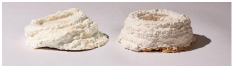
Figure 3: (A) First print attempt using the original printing formulation. (B) The print after adjustment of the formulation.
