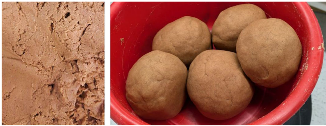
Fig. 3 Wood-CMC wet paste formed into lumps before loading (B1 formulation)
