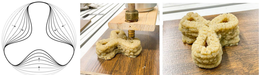
Fig. 4. (Left) Diagram, Development of a potential curvature tool path for encouraging cyanobacterial motility using CAD tools such as Rhinoceros and Grasshopper. (Right) Images, Robotic printing of the developed tool path with non-living sand-based mixtures towards printing with cyanobacteria.
