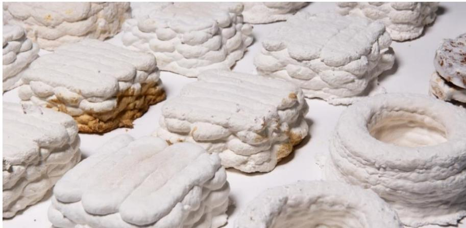
*Figure 6 - Printed models after full inoculation and drying.*
