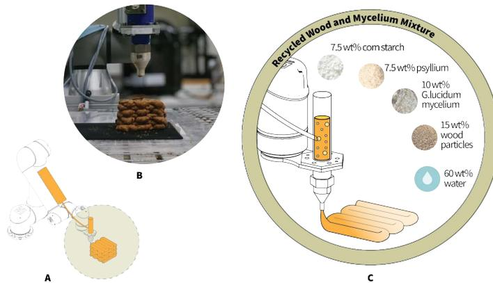
Fig. 3 - (A) 3D printed model toolpath; (B) Printed model using a 50% psyllium / 50% corn starch gelling agent ratio with the printing setup parameters; (C) The printed formulation
