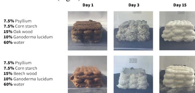
Fig. 4 - Surface colonization of mycelium on two wood types (beech and oak), 0.8 - 1.4 mm particles size, observed at 24 hours, 3 days, and 7 days.
