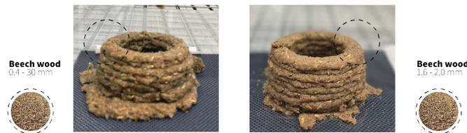
Fig. 5 -(A) The 3D-printed cylinder model using 0.4–30 mm particle; (B) printed with 1.6–2.0 mm particle sizes.
